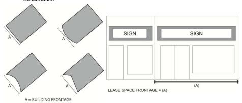
e. **Wall Area**: The wall area shall be calculated by the width of the exterior wall and height of the wall.
