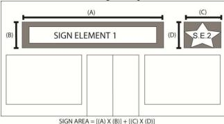
c. **Measurement of Signage on the Window**: The sign area is determined by calculating the area enclosed by the smallest single rectangle that will enclose the outside dimensions of the sign display.
