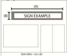
b. **Sign Area, Attached Sign (Multiple Elements)**: When signs are constructed of individual elements, the area of all sign elements, which together convey a single, complete message, shall be considered as a single sign. The sign area is determined by calculating the area enclosed by the smallest single rectangle that will enclose the outside dimensions of the background panel or surface, including sign trim or frame.
